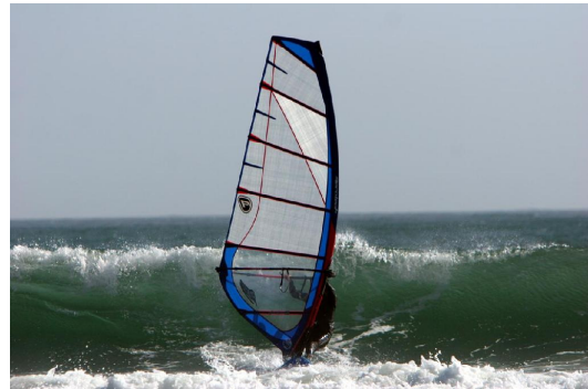
A sail made of Cuben, a loose-fill UHMWPE-reinforced mylar. Note how the loose fibres add haze and some loss of transmission. Before their acquisition by DSM Dyneema, Cubic Tech was working to market the fabric for use in airships. 381 Photo: WARDOG © SurfingSports.com, Inc.
