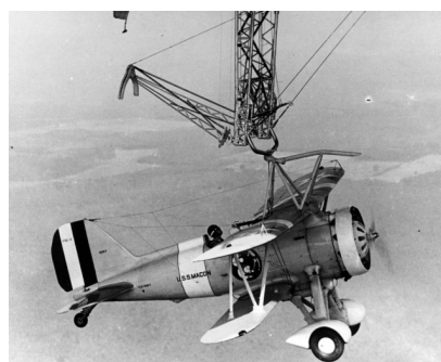
F9C-2 Sparrowhawk fighter docked with the airship USS Macon. The USS Macon and Akron served as airborne aircraft carriers in the 1930s. Photo: Naval History Center.
