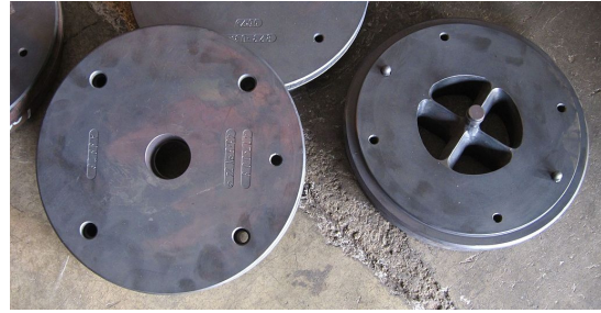
Tube extrusion die plates. The plate on the right blocks off the flow from the center, while the plate on the left subsequently constrains the exterior shape. Photo: Stephen Woolverton
