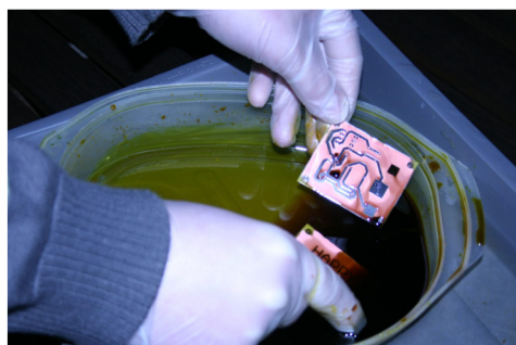
PCB etching with a ferric chloride solution. Photo: Adam Greig
