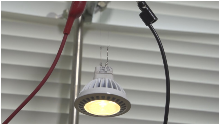
Carbon nanotube-based wire simultaneously suspends and illuminates a bulb. Photo: Rice University
