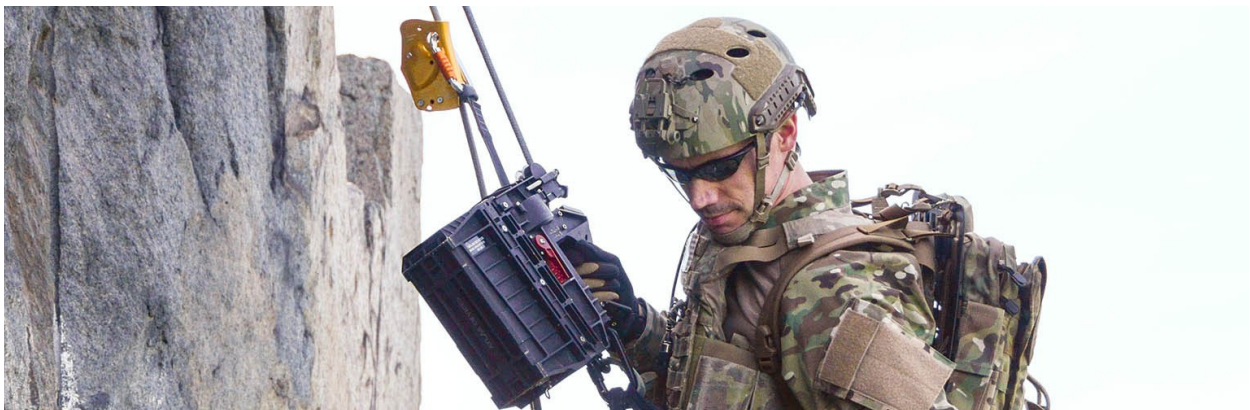
The Atlas APA-5 rope ascender weighs 9.1kg (including a swappable battery), lifts 270kg, can climb 213 meters per charge, and can be operated by remote control. 136 Photo: Atlas Devices
