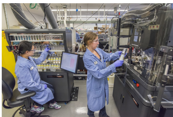
Overture, a robotic chemistry lab designed for protein synthesis applications. Photo: © 2010 The Regents of the University of California, through the Lawrence Berkeley National Laboratory.
