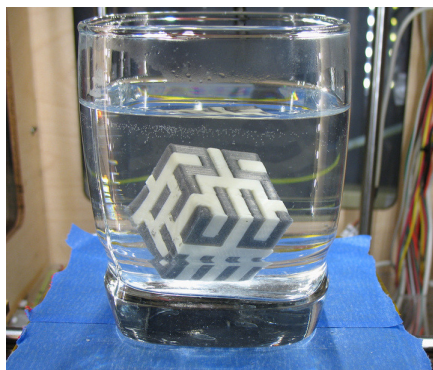
Hydrogel support dissolving away from a 3d print. Photo: Tony Buser
